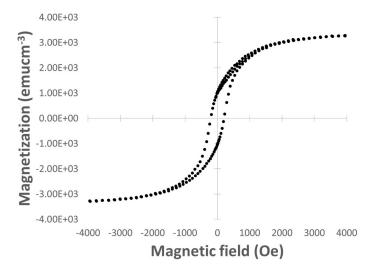
Magnetization M versus magnetic field, measured from the 40 nm thick FDLS at 300 K. For comparison, the saturation magnetization commonly reported for YIG is  $4\pi M$ =1750G=139emucm<sup>-3</sup>.
